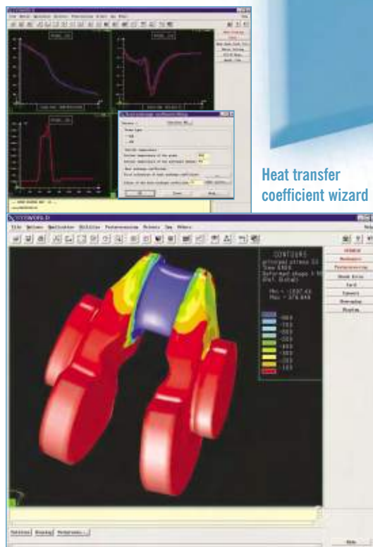
Compressive stresses displayed on the distorted structure
