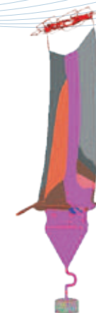
Prediction of stray crystals in SX part
