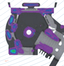
Application of pressure intensification The reduction in gas porosity due to the increased pressure can be identified with the simulation.
