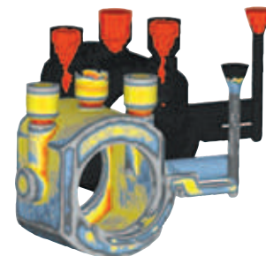
Pipe Shrinkage Prediction for a steel component
