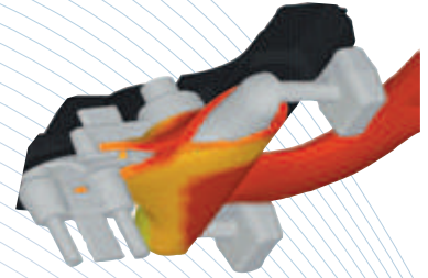
Metal Front Progression around a core
