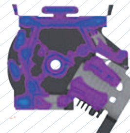
No pressure intensification Effect of piston pressure during the compression stage on the hydrogen porosity in an aluminum high pressure die casting component.
